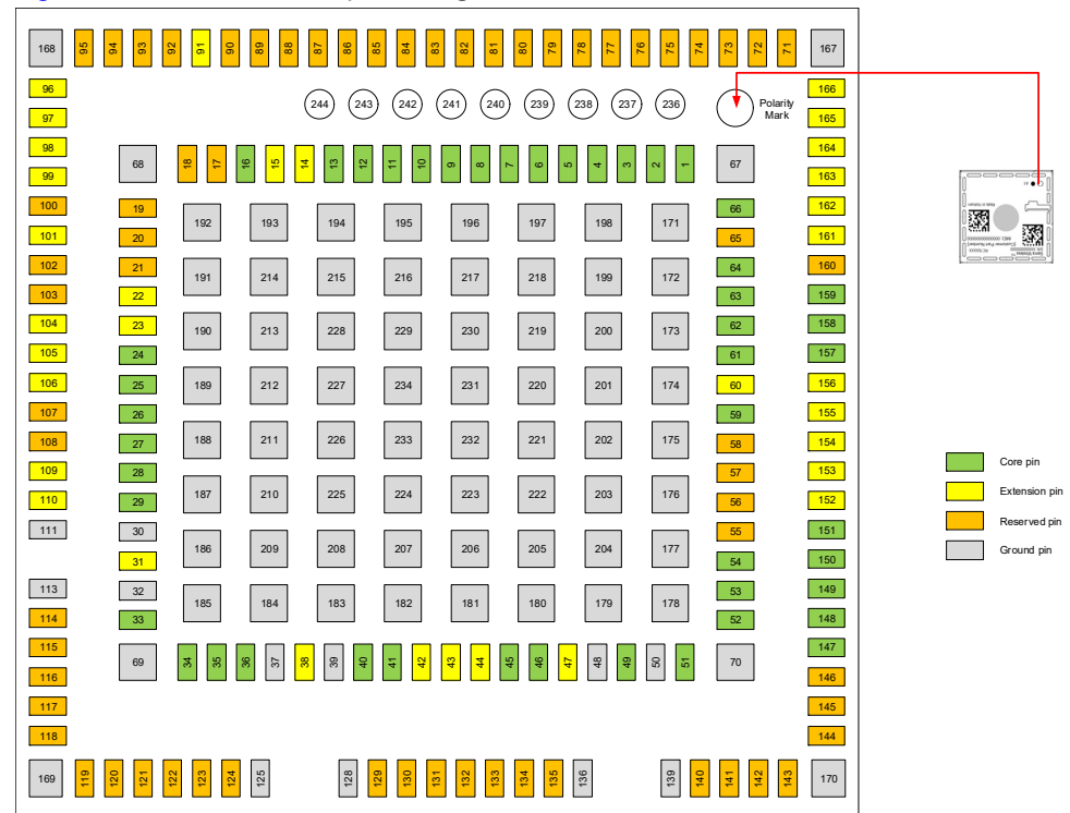
Figure 10-1: Pin Configuration (Top View, Through Module)
